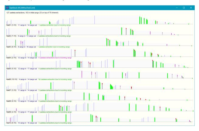
This time, the bright green (no container above the one needed) is nearly everywhere, while the bright read is quite scarce in the screenshot, illustrating the efficiency of placement of the incoming containers. Indeed, just 127 useless reshuffles/shifts were necessary to empty completely the storage area – as compared to the 191 obtained with even a reasonably good heuristic.
