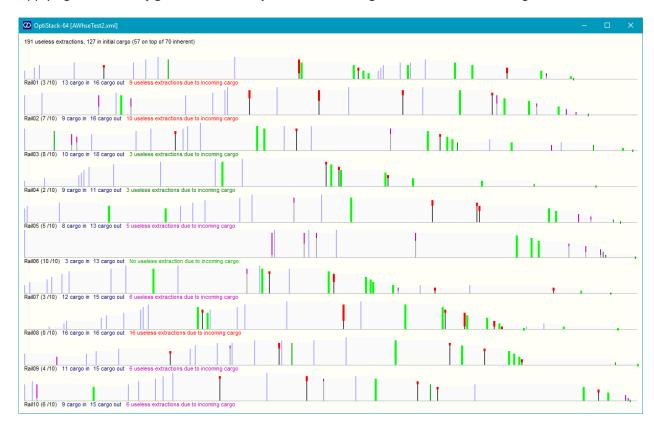
There is now significantly less bright red (and more bright green) in the screenshot, meaning quite fewer useless reshuffles/shifts of the containers in the Simulation. Indeed, only 191 useless extractions happen in that Simulation, compared to the 327 obtained with a random placement of incoming containers.
